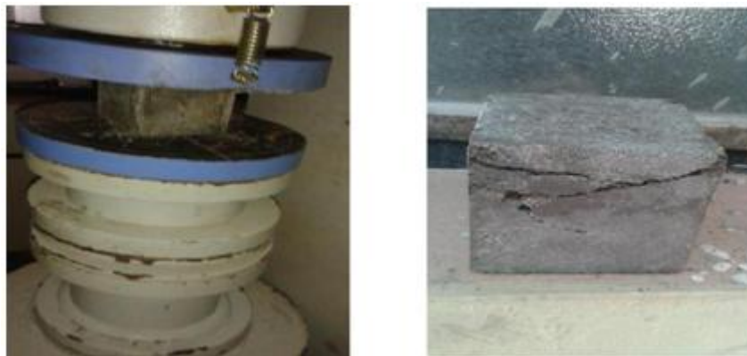
Fig. 4 Testing of mortar cube
