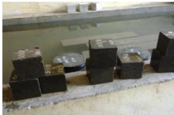
Fig. 3 Curing of mortar cube
